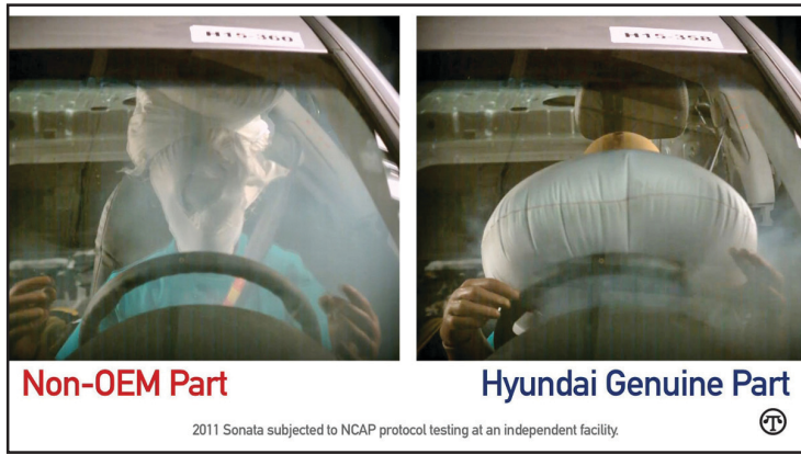
This test shows the difference between a non-OEM air bag and a Hyundai genuine air bag.
